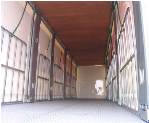
Above Left: The unique carpet sliding posts and plywood roof included on either side of the trailer. Above Right: Getting loaded at the dock!
