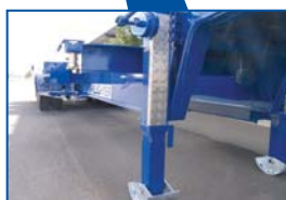
Aluminium Chequerplate provides long lasting protection for the landing legs
