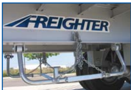
Heavy duty tyre carrier is designed to withstand the rigours of off road use
