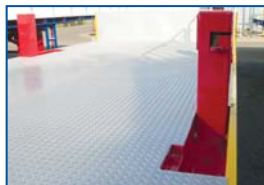
Fold-down twistlock pedestals are available on drop decks
