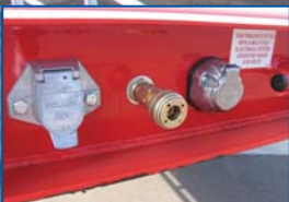
Road train rated wiring
