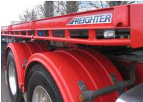
• 25mm NB pipe tie rails
