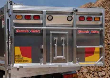
• Tailgate hinge configuration, operable from the ground
