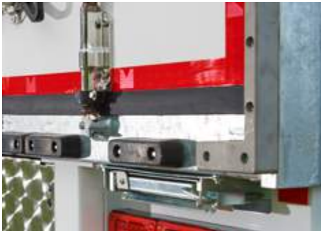
Stainless steel rear corner castings
