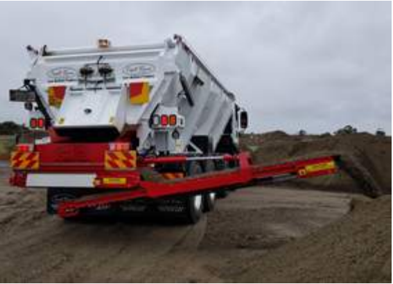
• Pivoting Side Conveyor Extends from 1.5m to 3m past the RH side of the body
