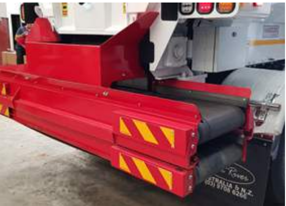
• Extendable Side Conveyor (horizontal) Extends out 1.5m past the RH side of the body
